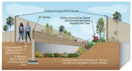
Figure 2 Conceptual Typical Cross-Section of Project's Channel Improvements (Looking Upstream)
