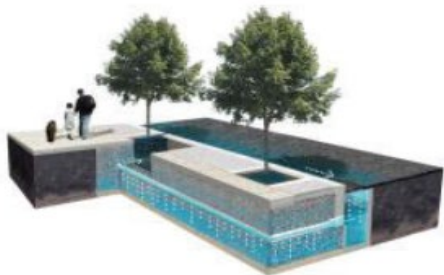
Bioretention Swale with Native Trees
