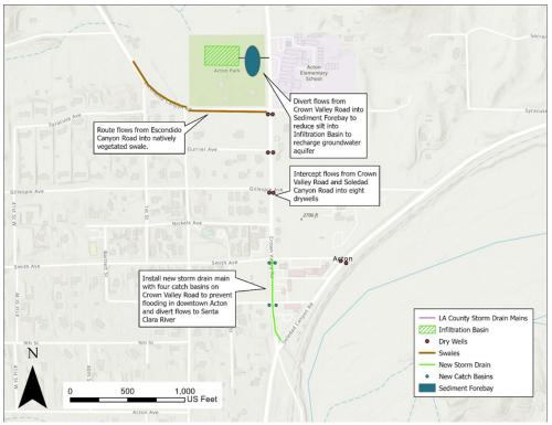
Figure 2. Proposed Stormwater Capture Improvements to Acton
