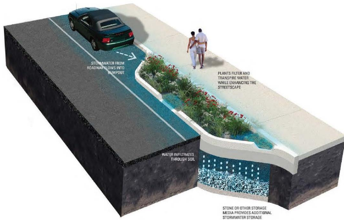
Mid-block Stormwater Bump-out
