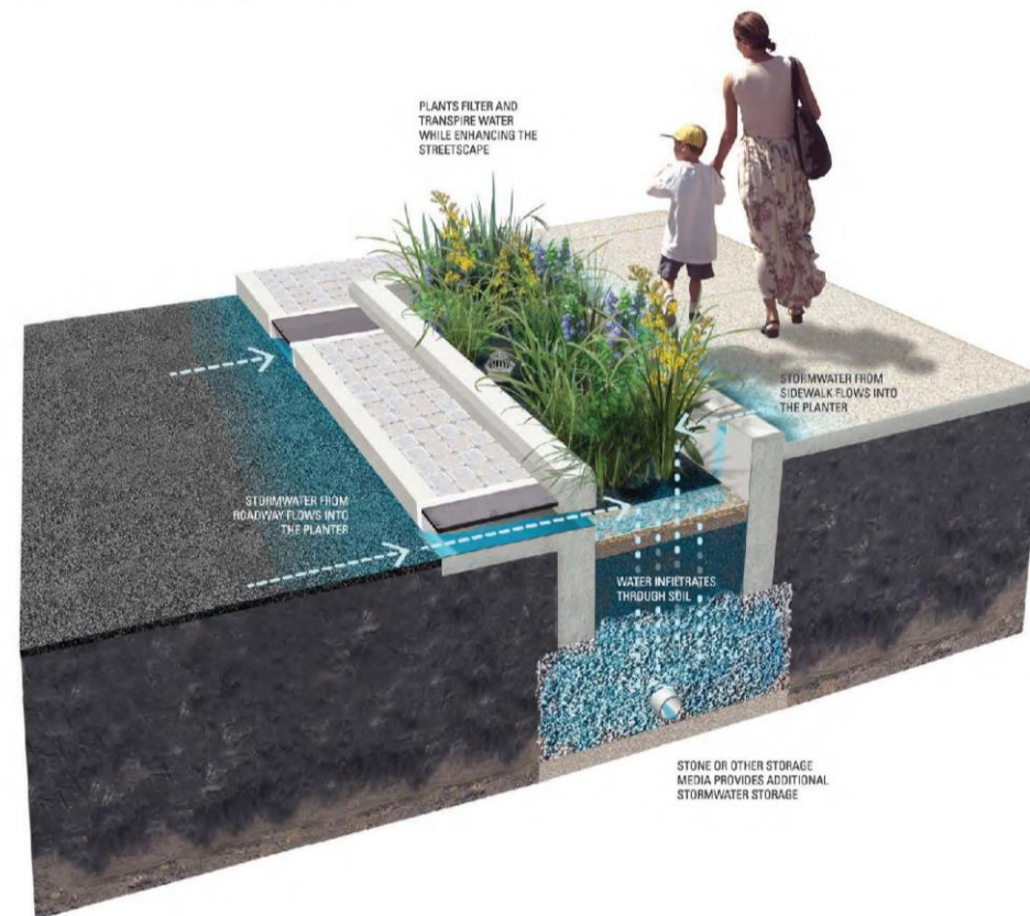
Figure 2.1: Three-Dimensional View of a Stormwater Planter
