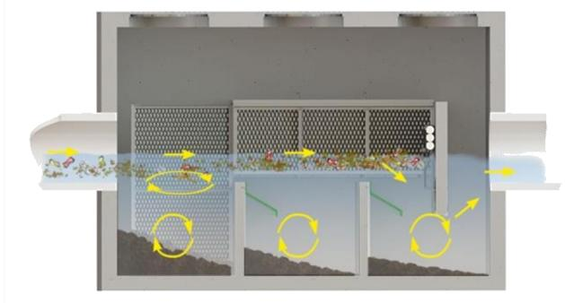
Pretreatment Device: remove pollutants/trash Figure 2.7: Three-Dimensional View of a Stormwater Drainage Well
