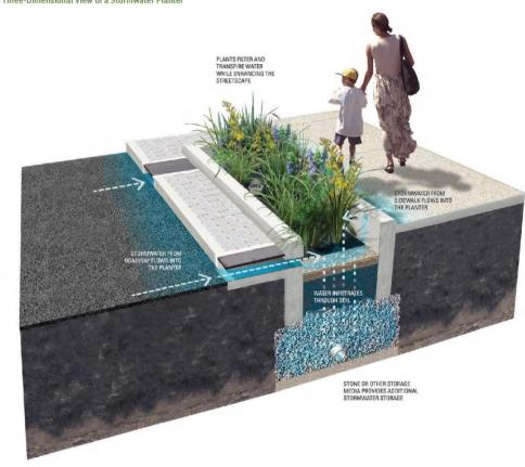
Figure 2.1: Three-Dimensional View of a Stormwater Planter
