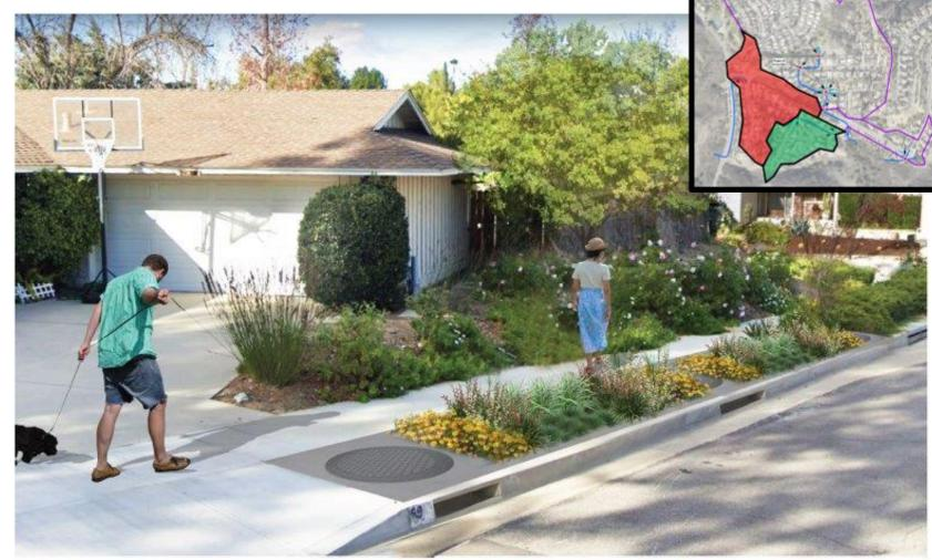
PERSPECTIVE VIEW STORMWATER BIOFILTRATION SYSTEM WITH 100% PLANTING AREA
