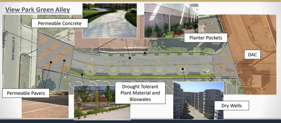
**Pre-Treatment** System Existing 45" Storm Drain **Green Alley** 36" diameter **Dry Wells**
